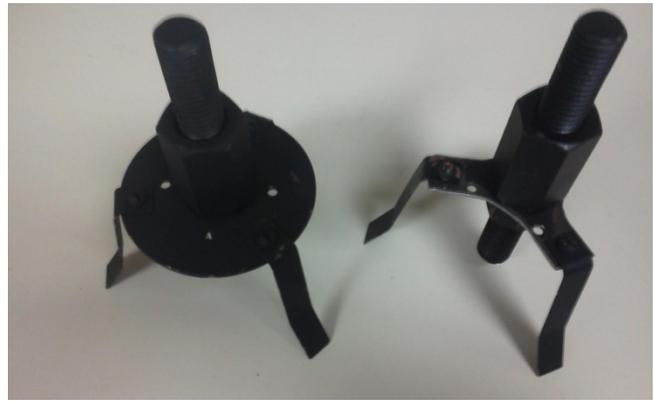
Figure 7. Original (left) and modified (right) flange-and-bolt assembly
