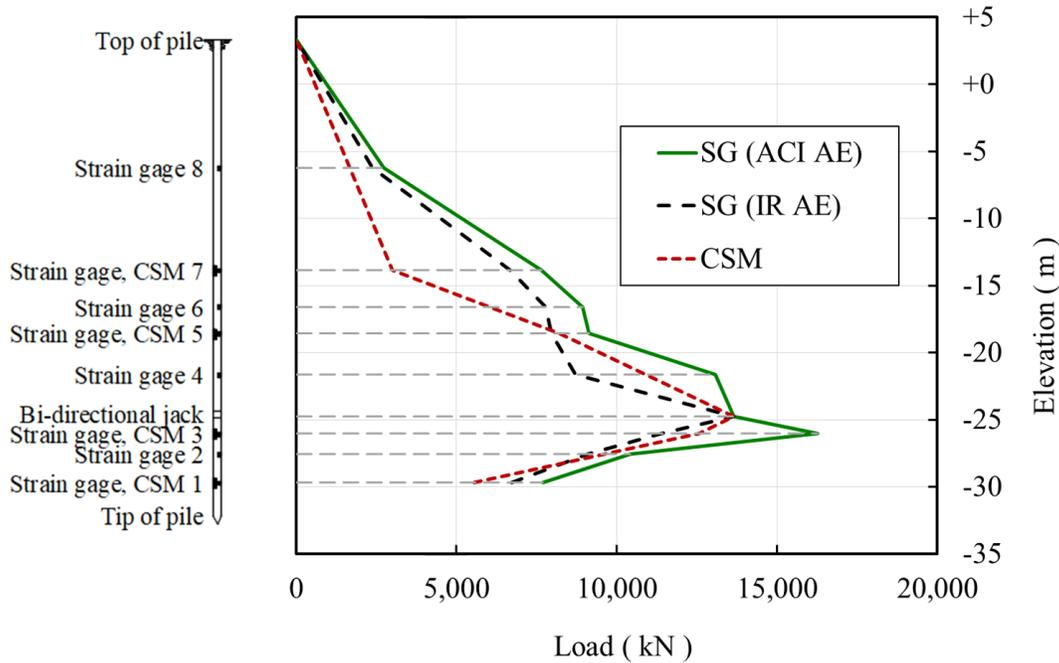
Figure 8. Pile elevation schematic and force distribution curves – Project B
