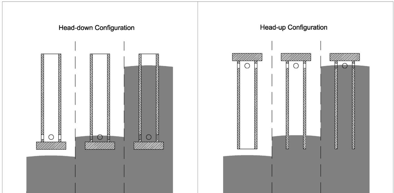
Figure 2. Modified self-filling CSMs being submerged in grout
