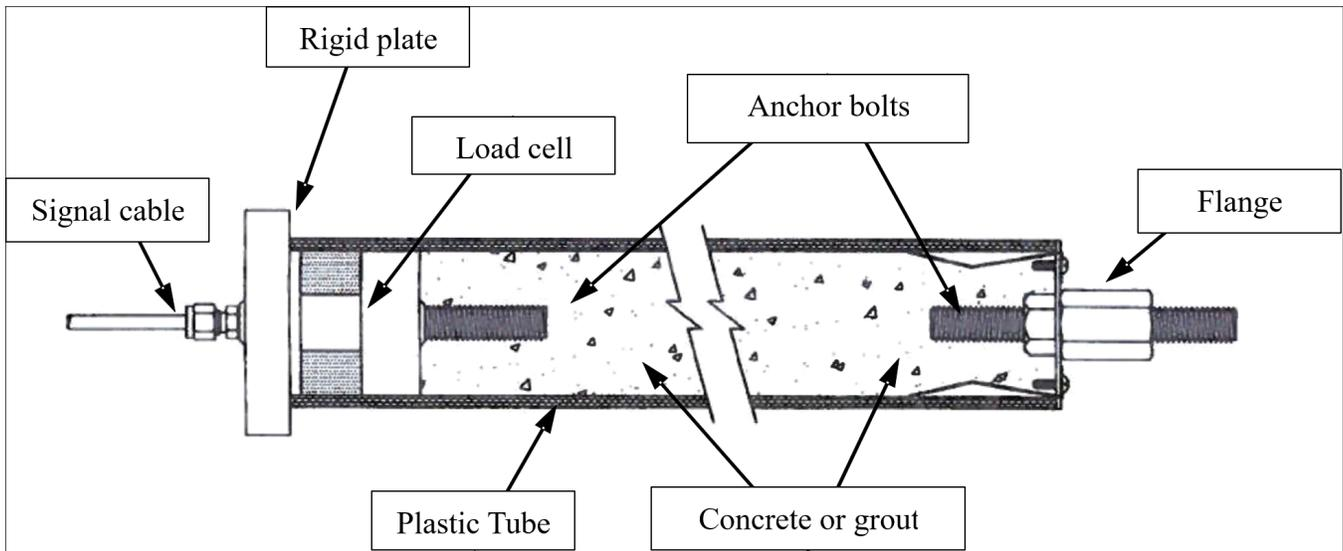
Figure 1. Concrete Stressmeter (after Geokon Inc.)
