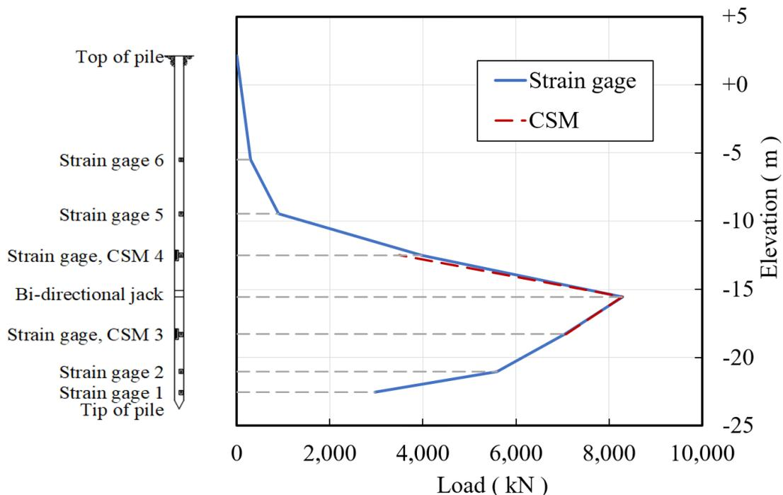
Figure 5. Pile elevation schematic and force distribution curves – Project A
